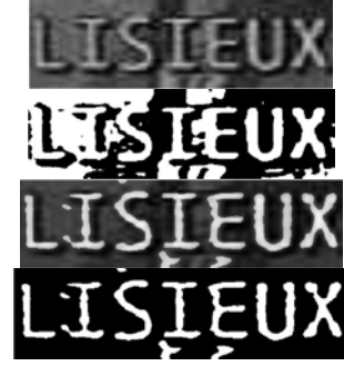
Figure 8 (a) original image, (b) binarization result of the image, (c) enhanced image using proposed method, (d) binarization result of the enhanced image
