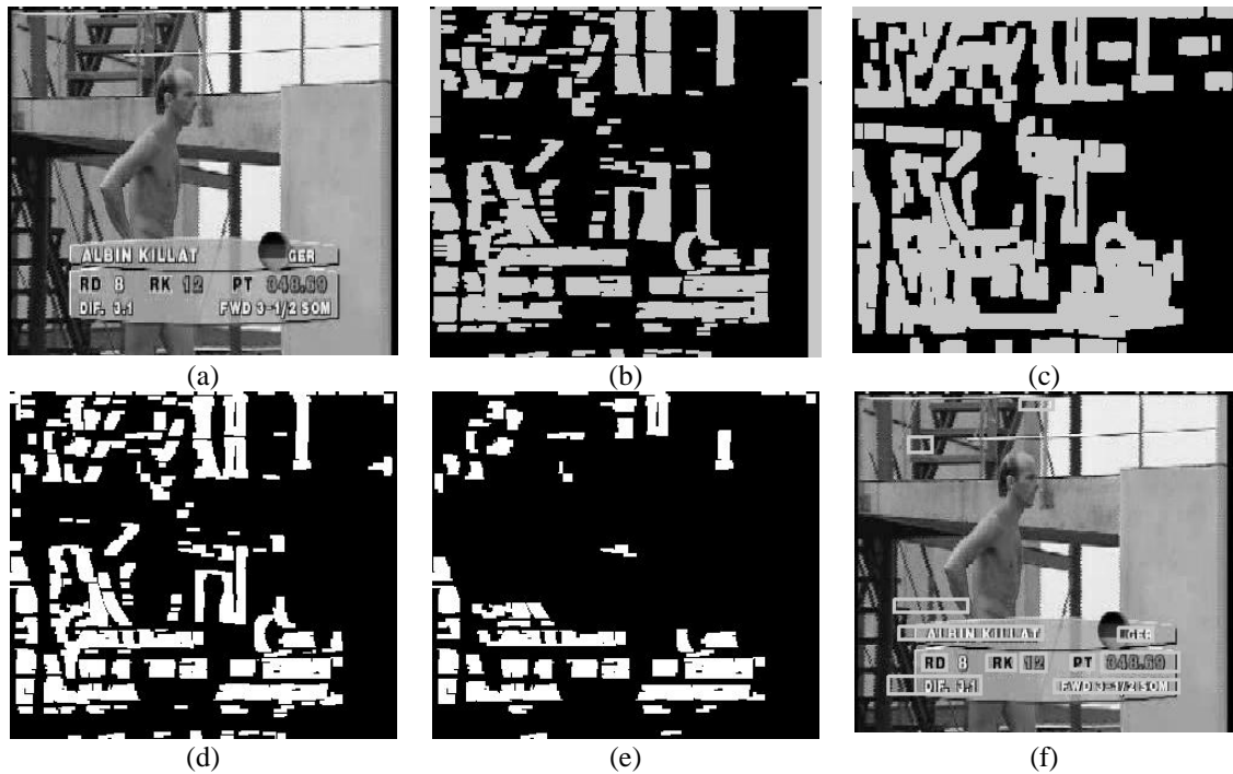
Figure 3 Candidate text region detection and text line location: (a) original image, (b) vertical edge dilation, (c) horizontal edge dilation, (d) integration of vertical and horizontal edge dilation, (e) updated regions after baseline location, (f) candidate text lines
