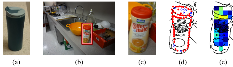
Fig. 8: Region information is necessary for robust shape recognition. The false positive shown aligns well to the edgemap but the interior matches poorly. (a) Model object. (b) False positive detection. (c) Zoomed in view of the false positive. (d) Edge points matched on top of the edgemap (red is matched, blue is not matched). (e) Activation scores of individual HOG cells [43]. Hotter color equals better match.
