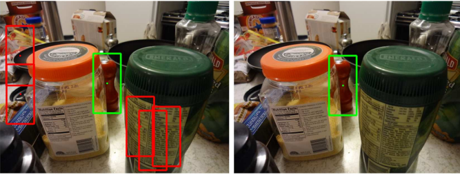
Fig. 14: A typical case where OCLP performs better than OPP. (left) For OPP, the false positives in red have higher scores than the true detection in green. The occluded region at the top of the true detection is over-penalized. (right) For OCLP, the true detection is the top detection.
