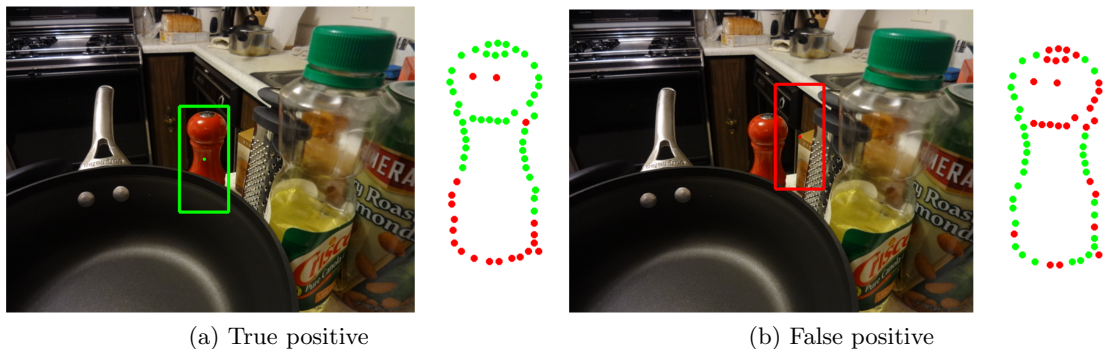
Figure 6.8: Examples of occlusion hypotheses. (a) For a true detection, the occluded markers (red) are consistent with our model. (b) For a false positive, the top of the object is hypothesized to be occluded while the bottom is visible, which is highly unlikely according to our model.
