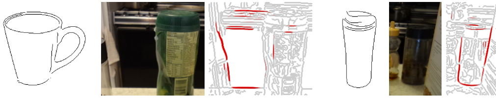
Figure 4.14: False positives of GN. Each triplet shows (1) template, (2) false positive window and (3) predicted match in red overlaid on the Canny edgemap.
