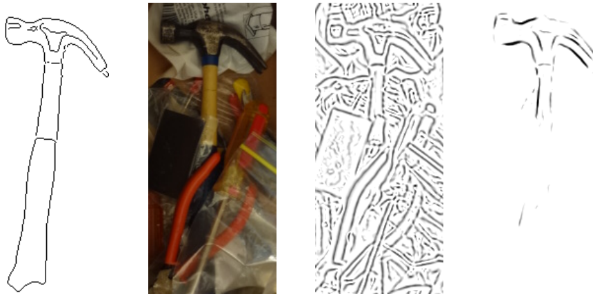
Figure 4.1: Example of shape matching under heavy occlusion. (left) Hammer template, (center-left) image window, (center-right) normalized gradient magnitudes, and (right) probability that each pixel matches the shape of the hammer.
