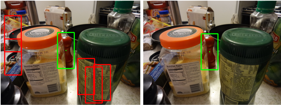
Figure 6.15: A typical case where OCLP performs better than OPP. (left) For OPP, the false positives in red have higher scores than the true detection in green. The occluded region at the top of the true detection is over-penalized. (right) For OCLP, the true detection is the top detection.
