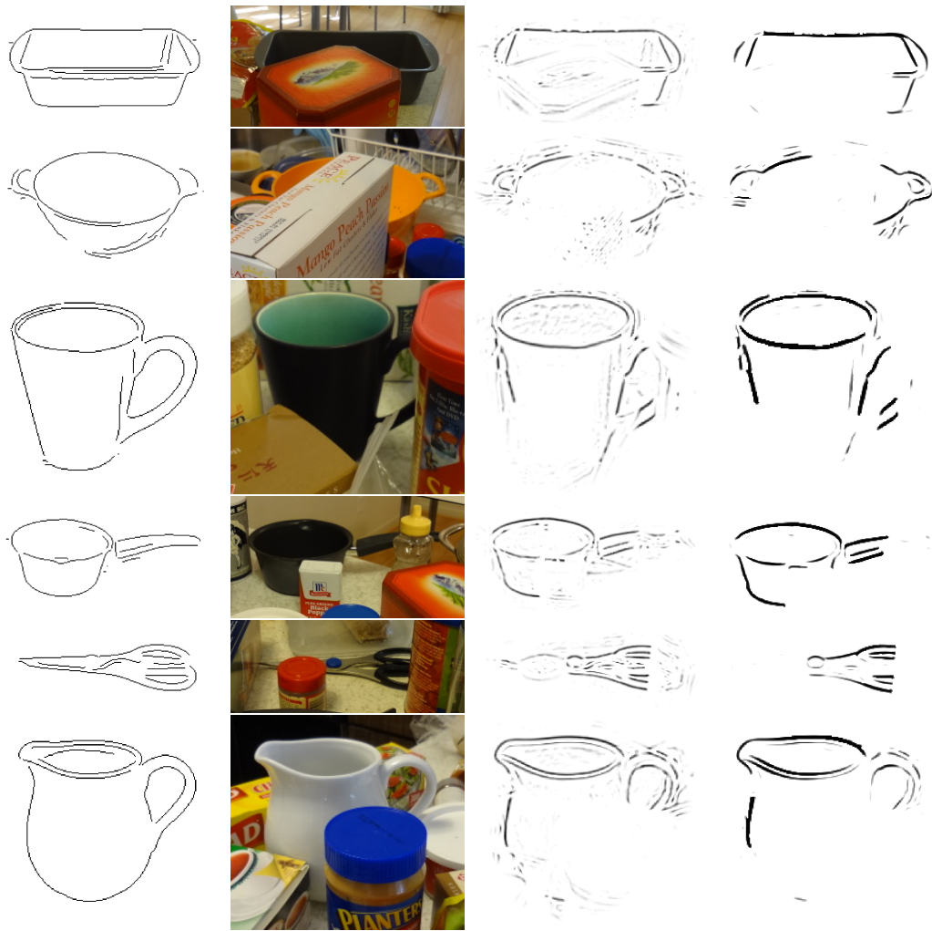
Figure 4.8: Results of shape matching using GN. From left to right, we show: 1) template, 2) window, 3) \Phi^S , and 4) probability that each pixel matches the template.
