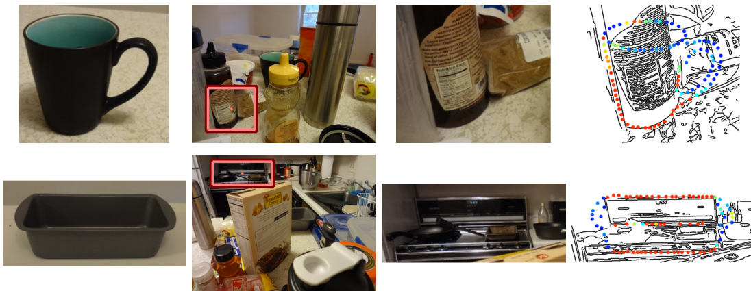
Figure 5.1: Example of false positives when using shape only. The edge information aligns well to the image but the interior does not match well. From left to right, we show (1) the model object, (2) a false positive detection, (3) the zoomed in view of the false positive, and (4) the edge points matched using Gradient Networks on top of the edgemap. The hotter the color, the better the match.
