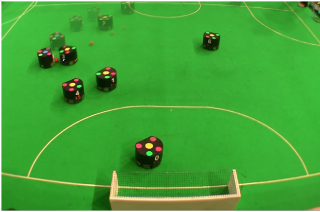
(a) Moving ball interception. Faded images show points along the trajectory of our robot, the ball, and a competing opponent robot.
