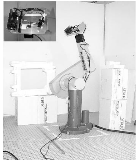
Figure 1: The experimental testbed for sensor-based MP. The sensor, a triangulation based area scan laser range finder, is mounted on the PUMA wrist. Inset shows an enlarged view of the sensor with the camera on the left and the laser striper on the right. See text for a complete explanation of the system.
