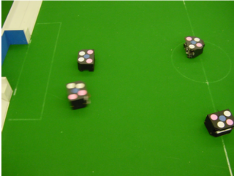
Figure 4: A robot (lower left) navigating through a field of static obstacles, using an RRT path planner. Color pictures and short movies are available at ftp://sponge.coral.cs.cmu.edu/pub/movies/F180-RRT/ .
