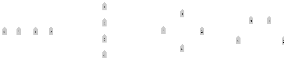
Fig. 3. Formations for four robots. From left to right: line , column , diamond , wedge . Each robot has a specific position to maintain in the formation, as indicated by its identification number (ID).
