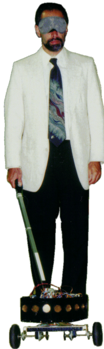
Figure 1: A blindfolded experimenter walks with the GuideCane.
