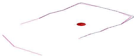
Figure 6: Environment maps derived from the first and second snapshots using recursive line fitting. The Nomad 200 mobile robot moved 5 inches to the right between the snapshots. (Red: first snapshot. Blue: second snapshot.)
