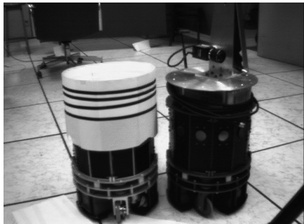
Figure 1: Robots used in the experiments. The leader robot (Rosie), is on the left while the follower (Agamemnon) is on the right. The upper part of Rosie has been covered with a pattern which is used to communicate to Agamemnon.
