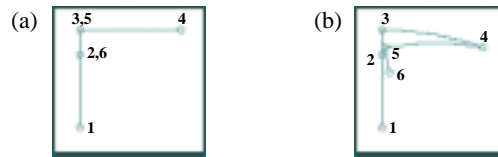
Figure 2: Illustrative example. (a) A path taken by the robot, along which it observed six indistinguishable landmarks (in the order of the numbers). (b) The robot’s odometry yields erroneous readings between the third and the fifth landmark observation.
