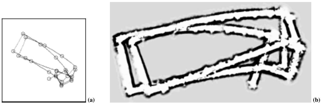
Fig. 3. (a) Raw data (2,972 controls). The box size is 90 by 90 meters. Circles indicate the locations where landmarks were observed. The data indicates systematic drift, in some of the corridors. The final odometric error is approximately 24.9 meter. (b) Occupancy grid map, constructed from sonar measurements using the raw odometry data.
