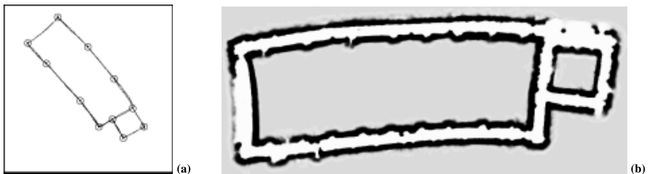
Fig. 4. (a) Maximum likelihood map, along with the estimated path of the robot. (b) Occupancy grid map constructed using these estimated locations.
