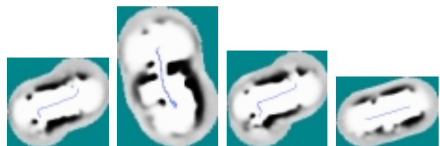
Fig. 7: Examples of local maps, annotated by robot trajectories. These maps have been constructed from sonar measurements.
