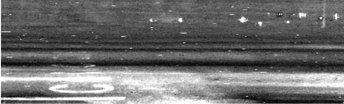
Figure 4-15. A laser intensity image taken in a parking lot. Intensity should decrease monotonically as distance increases. Instead the intensity on the ground appears to oscillate as the distance increases. The banding along the ground is caused by optical crosstalk and occurs at approximately 6.5 meter intervals, the ambiguity interval of the high frequency modulation channel of the laser. At the left of the image, the white stripes with the sideways 'C' in-between them is a parking space ('C' stands for compact).
