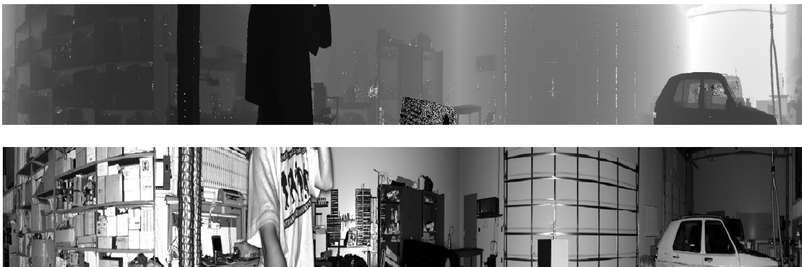
Figure 4-8. Range and reflectance images taken in our lab with the scanner using the Z+F laser. We have subsampled each of the images in the horizontal direction by a factor of 3 to make them fit on to the page. In the range image, top, darker pixels are closer and brighter pixels are farther. The range values have been scaled for printing so that a range of 14 meters or more appears as white. In the reflectance image, bottom, brighter pixels correspond to points of higher reflectance. The reflectance values have been scaled for better printing as well.
