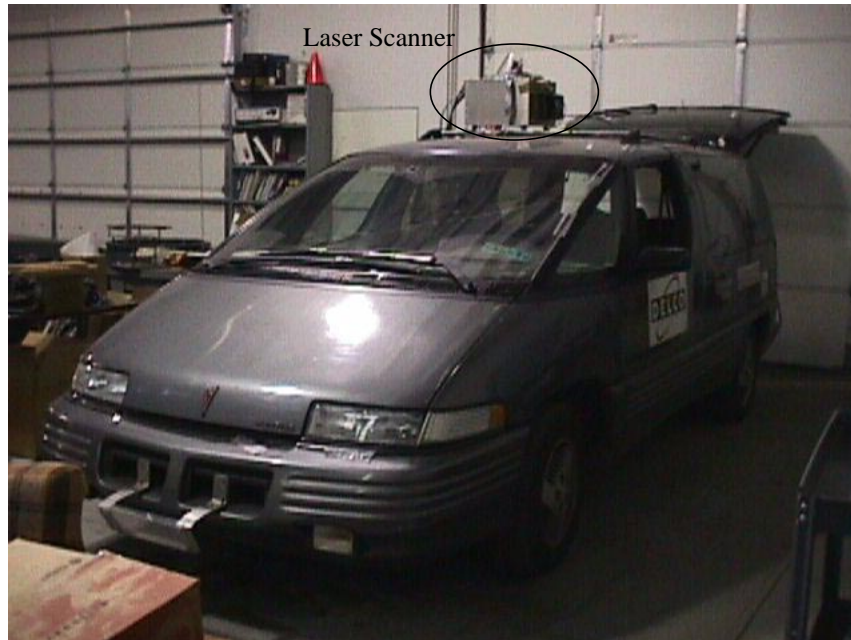
Figure 1-1. The testbed for the thesis work. The laser scanner built by K2T and Zoller and Fröhlich is mounted on the roof of Navlab 5, one of Carnegie Mellon's automated vehicles.
