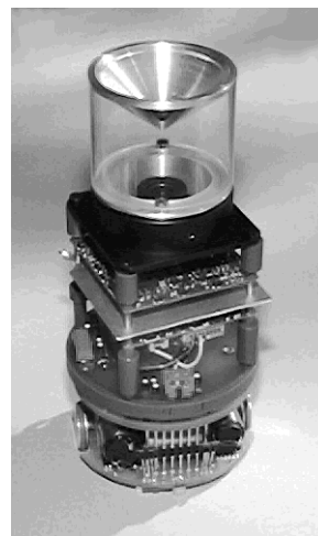
Fig. 2. Khepera TM robot with camera module and custom made conical mirror, which permits sampling of the environment over 360°, in a range of ±10° about the horizon.
