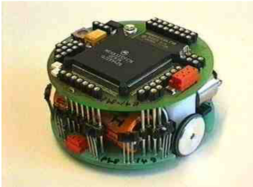
Figure 3: The Khepera Robot (diameter 6 cm).
