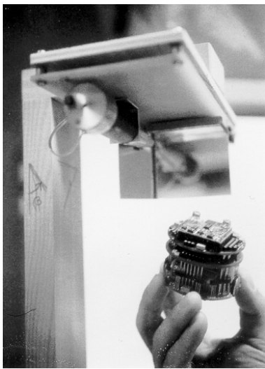
Fig. 3. A close view of the robot with the “helmet” for capturing laser signals and the laser device on the background.
