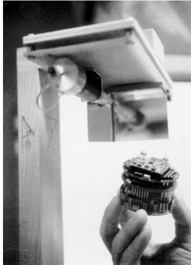
Figure 2: A close view of the robot with the "helmet" for capturing laser signals and the laser device on the background.
