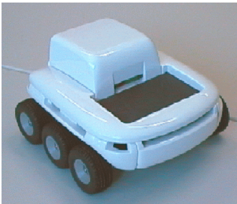
Figure 7. Koala , the big brother of the famous Khepera robot, developed by the swiss company K-Team S.A. Its size is about 30x30 cm.
