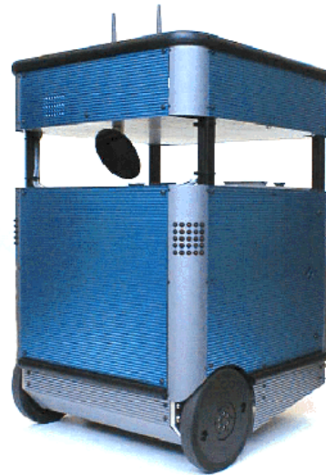
Figure 8. Pygmalion is a sophisticated and very powerful mobile robot for indoor applications. It sizes about 40x40 cm and has a height of about 50 cm.
