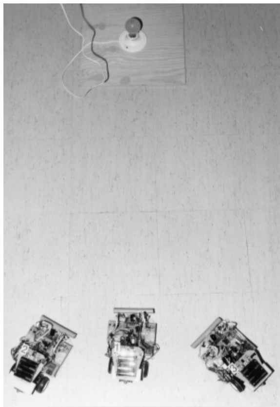
Figure 6: Initial configuration of three box-pushing robots before sensing the box at the top of the picture.
