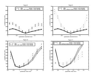
There is a tradeoff between robustness to systematic movement error and systematic vision error. SRL and MCL with noise favor robustness to movement errors while MCL without noise favors robustness to vision
