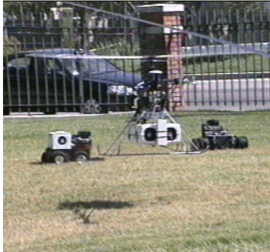
Figure 1. The experimental testbed consisting of the AVATAR (Autonomous Vehicle Aerial Tracking And Reconnaissance) robot helicopter and two Pioneer AT mobile robots
