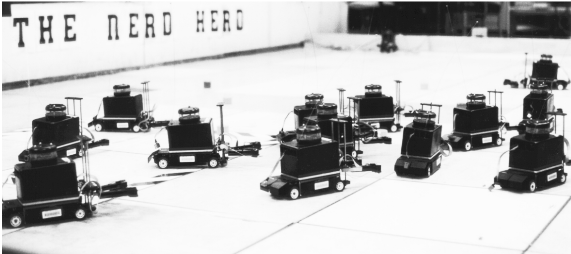
Figure 1-5: Some of the 20 mobile robots used to validate the group behavior methodologies described in the thesis. These robots demonstrated group safe-wandering, following, aggregation, dispersion, flocking, and foraging.
