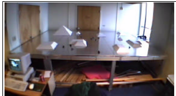
Figure 2: The microrobotic environment. The white pyramids are moveable obstacles. The little black dots are the robots.
