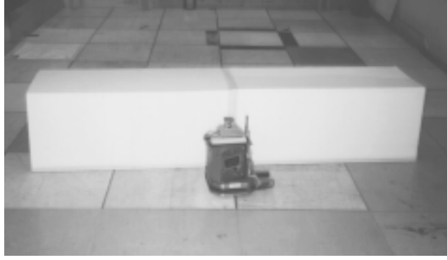
Fig. 5. Fault tolerant action selection. In the first experiment, we seize one of the R-2 robots and turn it off. This causes the remaining R-2 robot to have to perform both tasks of the box pushing mission: pushing at the right end of the box, and pushing at the left end of the box. Here, the R-2 is acquiring the right end of the box.
