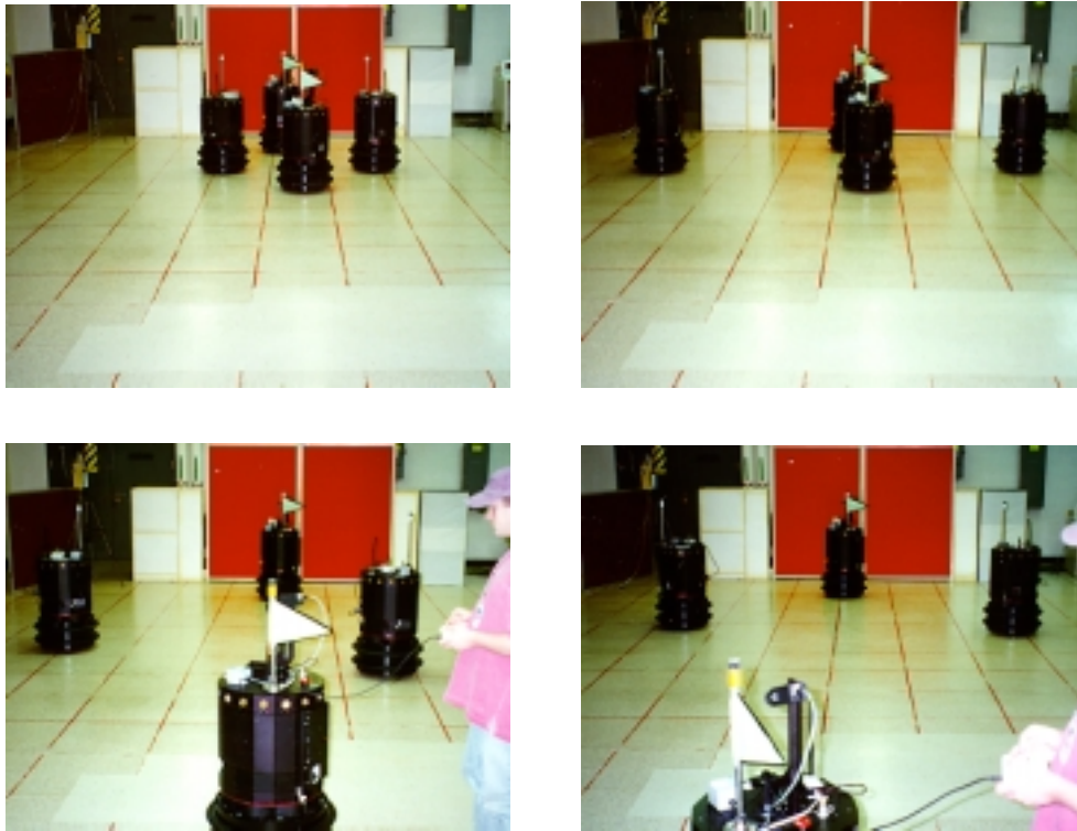
Figure 9: Results of robot team performing task using summation of force vectors. The robots with the triangular flags are acting as targets, while the robots without the flags are performing the distributed observation.
