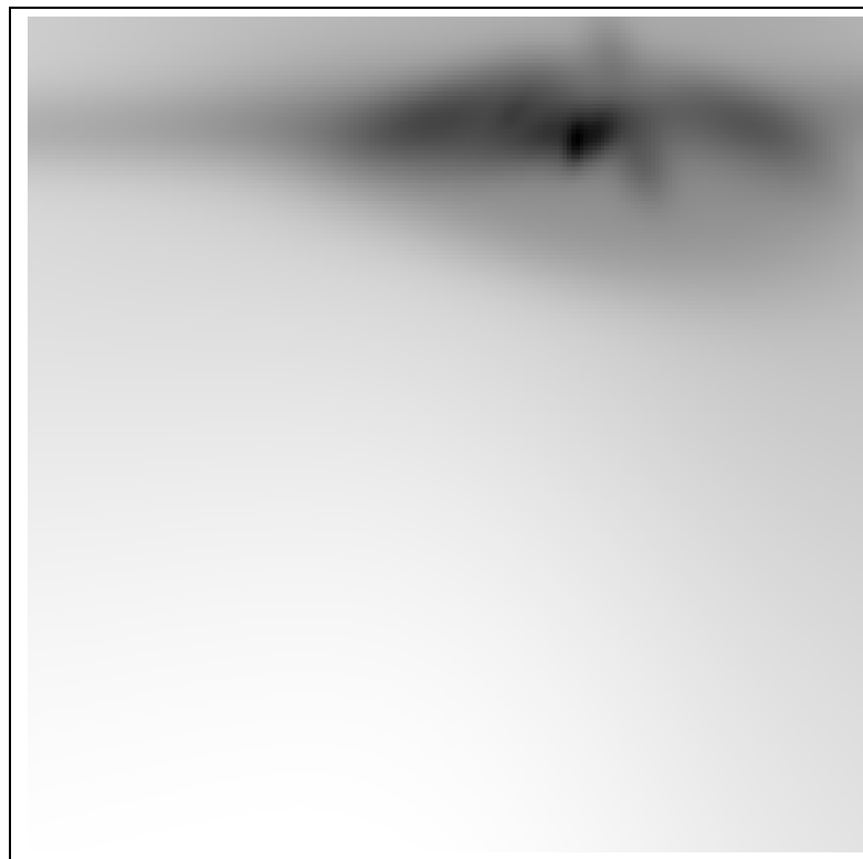
Figure 6: Laboratory scene and probability density function of robot pose. The area depicted corresponds to the 2 - D configuration space of the robot. Darker regions correspond to more likely poses, given the image.
