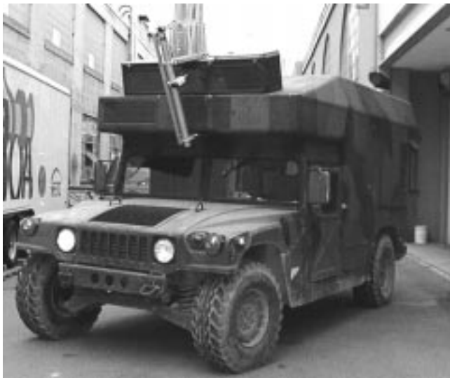
Fig. 13. The autonomous vehicle (HMMWV) used for our experiments. The vehicle is equipped with stereo vision, inertial guidance and GPS positioning.
