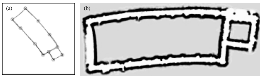
Figure 5. (a) Raw data (2,972 controls). The box size is 90 by 90 meters. Circles indicate the locations where landmarks were observed. The data indicates systematic drift, in some of the corridors. The final odometric error is approximately 24.9 meters. (b) Occupancy grid map, constructed from sonar measurements.
