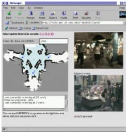
Figure 6: Web control interface. Users can log in on the left side of the window, and specify target locations by clicking in the map. The map shows current robot position, pending target locations, and a dialogue box displays the current speed of the robot. On the right, users can watch images recorded using the robot’s camera (top image) and by a stationary camera with zoom mounted on a pan/tilt unit (bottom image).
