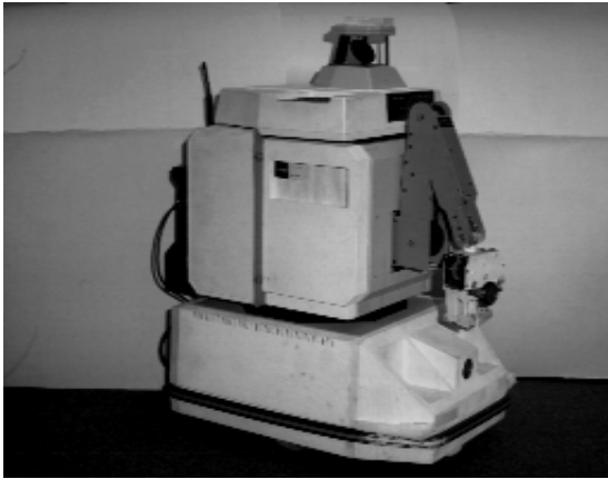
Figure 1: (a) COLUMBUS is a wheeled HERO-2000 robot with a manipulator and a gripper. It is equipped with a sonar sensor on the top of the robot that can be directed by a rotating mirror to give a full 360^\circ sweep (24 values). Sonar sensors return approximate echo distances. Such sensors are inexpensive but very noisy. (b) COLUMBUS explores an unknown environment. Note the obstacle in the middle of the laboratory. Our lab causes many malicious sonar values, and is a hard testbed for sonar-based navigation. For example, some of the chairs absorb sound almost completely, and are thus hard to detect by sonar.
