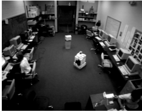
Figure 1: (a) COLUMBUS is a wheeled HERO-2000 robot with a manipulator and a gripper. It is equipped with a sonar sensor on the top of the robot that can be directed by a rotating mirror to give a full 360^\circ sweep (24 values). Sonar sensors return approximate echo distances. Such sensors are inexpensive but very noisy. (b) COLUMBUS explores an unknown environment. Note the obstacle in the middle of the laboratory. Our lab causes many malicious sonar values, and is a hard testbed for sonar-based navigation. For example, some of the chairs absorb sound almost completely, and are thus hard to detect by sonar.
