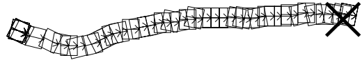
Figure 5: Sample trace of the execution of the reactive control algorithm. The target point is marked with a cross.
