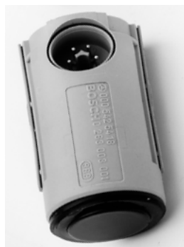
FIG. VIII. SINGLE ULTRASONIC SENSOR USED WITHIN AN ARRAY COMPRISING A MAXIMUM OF 8 SENSORS.
