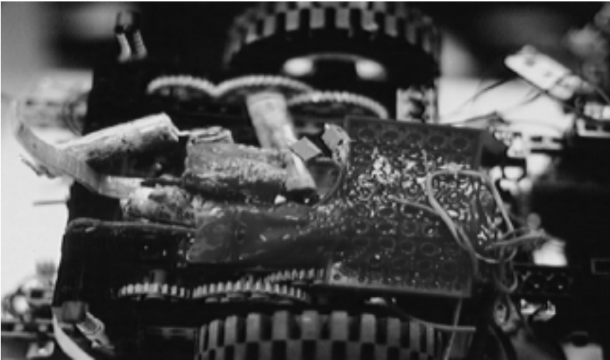
Figure 4: exploded battery-pack due to overcharge
