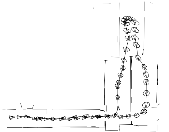
Fig. 8. Estimated robot location and built map using laser.
