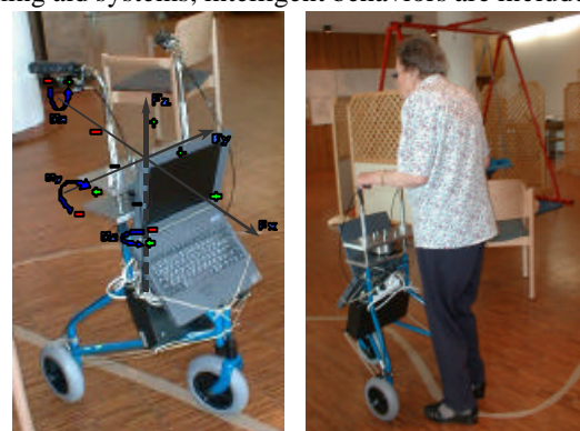
Figure 6. Test platform for force and torque measurements
