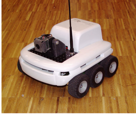
Fig. 5. The Koala robot, despite its look and size (31 x 32 x 18 cm), has operating features similar to those of the Khepera robot.
