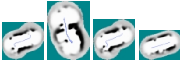
Figure 6: Examples of local maps, annotated by robot trajectories. These maps have been constructed from sonar measurements.
