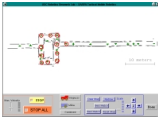
Fig. 7. Combined maps of Vespucci and Milka provides the complete picture that was not available to individual robots.
