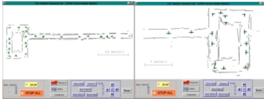
Fig. 6. Map built by Vespucci (left), starting from the West wing of the building. The second map was built by Milka (right), which started from the East wing of the building.
