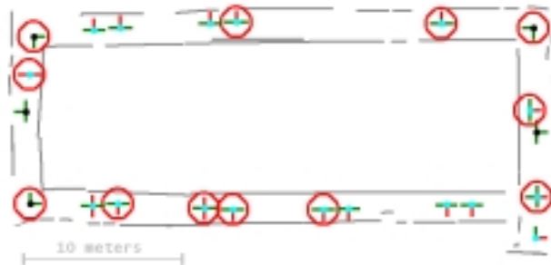
Fig. 4. Maps D_7 and D_9 of the same environment are matched against each other and their combination is correctly generated. Circles indicate features that were registered in both maps.
