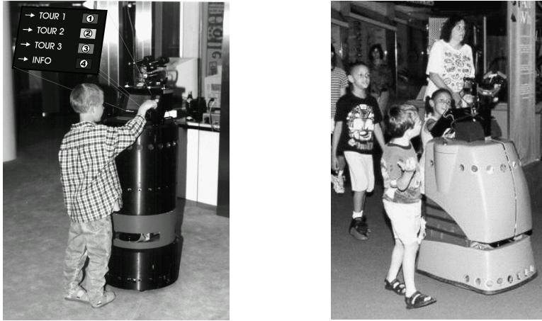
Figure 3: Two of the robots used for testing: RHINO (left) and MINERVA (center and right), which successfully guided thousands of people through crowded museums.
