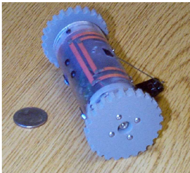
Figure 1: An assembled scout, ready for operation (shown next to a quarter for scale).
