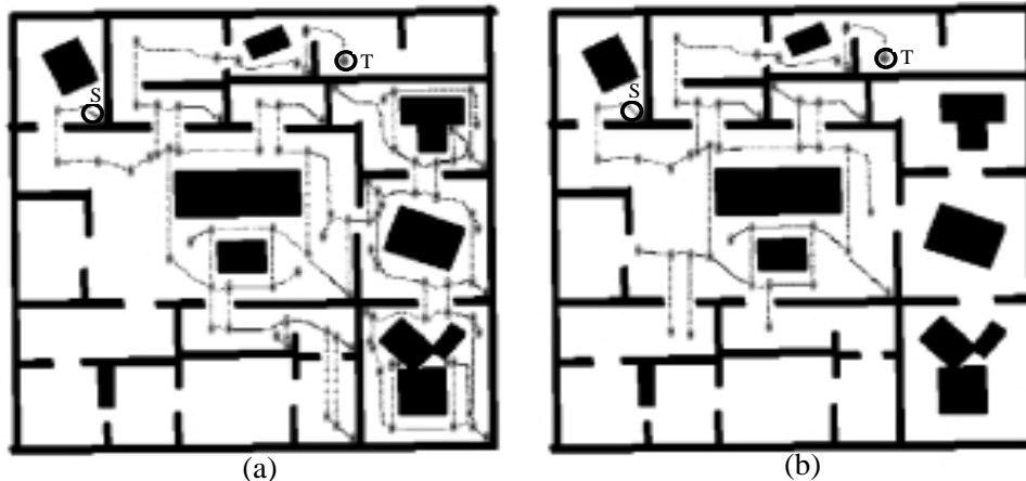
Figure 8: The roadmap generated by the searching robot in an office floor environment, using (a) Local-A* , and (b) Roadmap-A* . (Using a horizontal sweep direction.)
