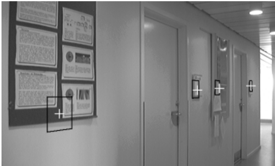
Fig. 2.: Locations of four landmarks detected using normalized cross-correlation after performing perspective re-mapping of the stored landmark pixel data, (figure 1). The white crosses are the loci of maximum correlation coefficient.
