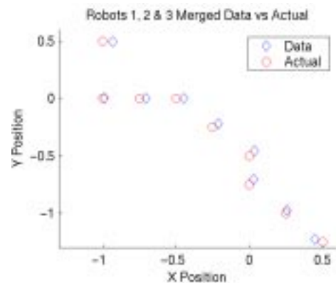
Figure 11. Trajectory produced by merging observations of robots 1, 2 and 3 (diamonds) compared to actual ball trajectory (circles). Notice further improvement in upper left.
