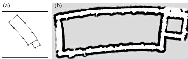
Figure 4: (a) Maximum likelihood map, along with the estimated path of the robot. (b) Occupancy grid map constructed using these estimated locations.
