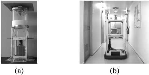
Figure 1. (a) Omni-directional camera. (b) Camera mounted on a Labmate mobile robot.
