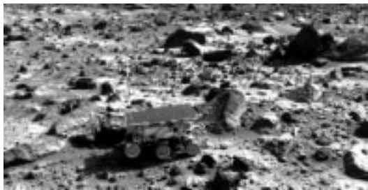
Figure 1: Typical terrain encountered on Mars by the Sojourner rover. The intrepid mobile explorer is 68cm long by 48cm wide, and stands 28cm tall.
