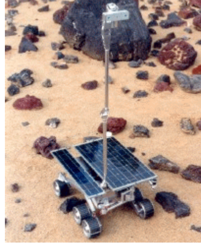
Figure 7: The Rocky7 Prototype Microrover, developed at JPL to test technologies for future missions. It is pictured here in the JPL MarsYard, an outdoor testing arena featuring simulated martian terrain.
