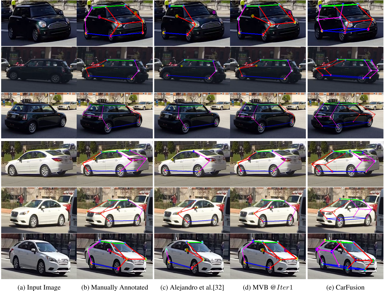
Figure 3: Qualitative analysis of the structured point detector before and after multiview bootstrapping (MVB), shown for two cars in three different views. Initial detectors were trained using Alejandro et al.[32]. The CarFusion approach was used to reconstruct the cars. Then the resulting 3D structured points were re-projected to all the views and used to retrain/bootstrap the detectors. The MVB approach shows clear visual improvement over the baseline, even in the presence of occlusions.
