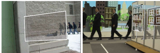
Figure 1: By using a 2D projective invariant to transfer image data between cameras, our system can render views of dynamic occluded objects in real time. As shown in these simulated multiple exposure images, our method creates videos that are accurate and convincing.
