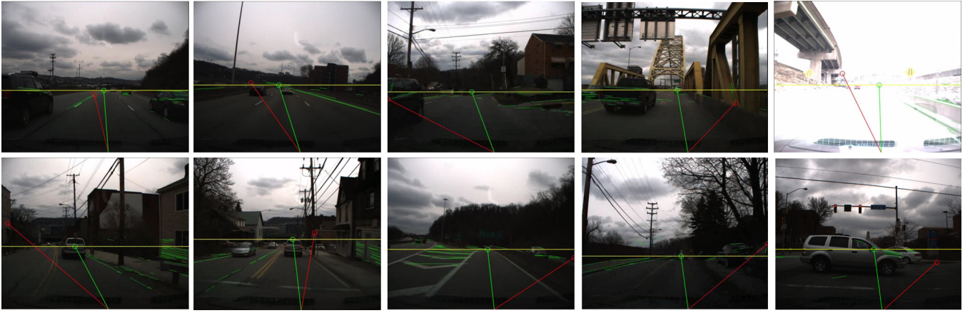
Fig. 4: A comparison of vanishing point locations by the frame-by-frame detection and by the EKF tracking.
